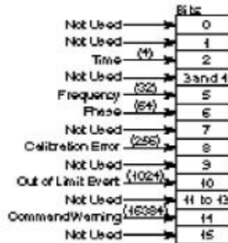
Figure 4-3. The Questionable Data/Signal Status Register Group
